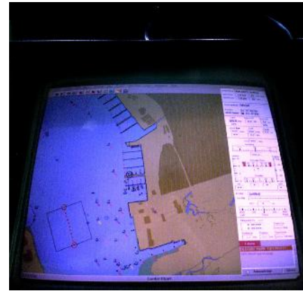
The ECDIS digital navigational charting system is a critical navigation tool in modern ships. LOS ANGELES TIMES VIA GETTY IMAGES
